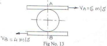
(c) Two wheels are attached to ends of rod AB as shown in figure No.11. [6] Determine angular velocity of rod AB and velocity of end B.
