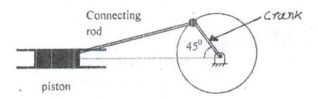
c) At the position shown in figure, the crank AB has Angular velocity of 3rad/sec clockwise. Find the velocity of slider C and the point D at the instant shown. AB=100mm. [06]
